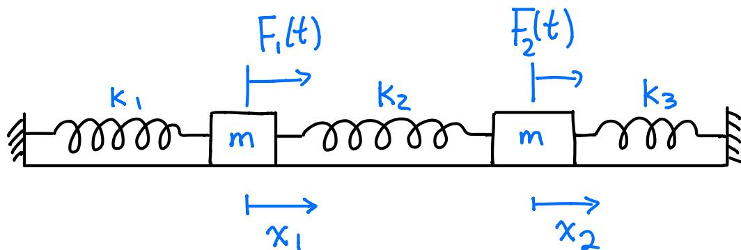
$$\begin{aligned} m \frac{d^2x_1}{dt^2} &= -k_1 x_1 + k_2 (x_2 - x_1) + F_1(t) \\ &= -(k_1 + k_2)x_1 + k_2 x_2 + F_1(t) \end{aligned}$$
