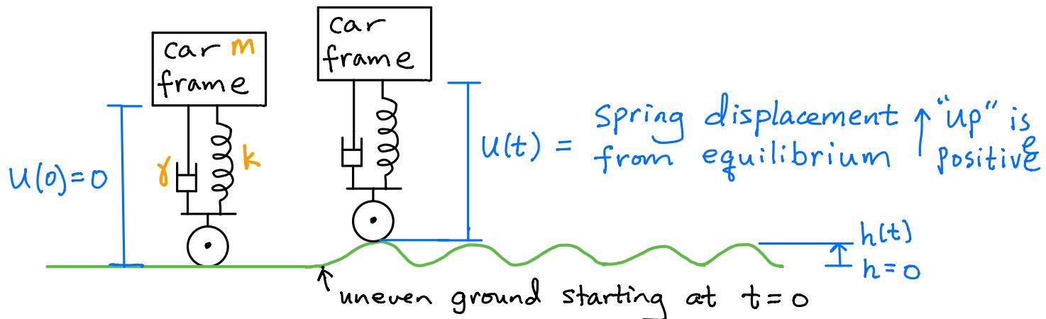
$$m(\text{car frame acceleration}) = -Ku - \gamma u'$$
