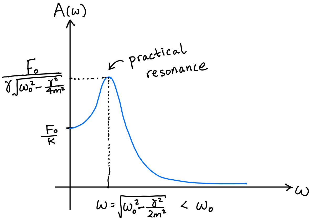
By adjusting damping  $\gamma$ , can change resonance frequency.
